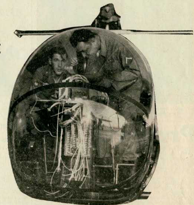
Personnel of the Avionics Detachment at the Etain Air Base, a TASCOM unit, install radio equipment in an H-13 helicopter. Army aircraft from all over Europe is flown into the installation to have special electronic equipment installed or repaired.
