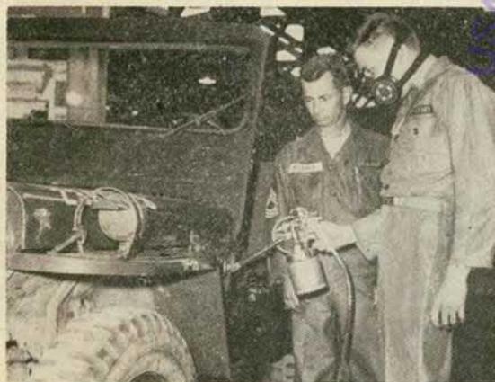
Keeping vehicles in a constant state of readiness requires painting and repair. Maintenance personnel in TASCOM Depots perform this important function so equipment may be sent to combat units in fully operational state. Here a jeep is being repainted at a TASCOM Depot in France before sending it to a unit in Germany.
